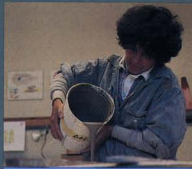
2. Pouring slip into plaster mold.
