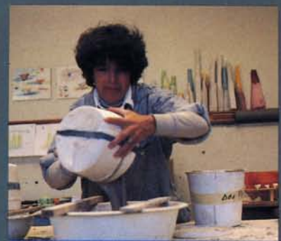
3. Draining excess slip from mold.
